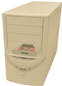
IDE to SD Adapter mounted onto 3.5" drive bay
