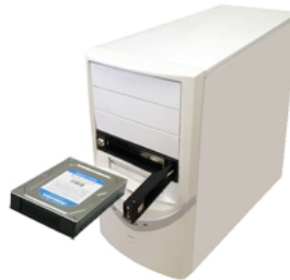
Snap-in 2.5" installed into Sanp-in SATA Mobile Rack
