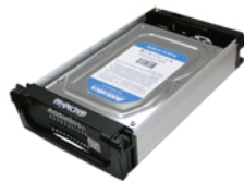
Snap-in 2.5" installed into a Diamond SATA drive enclosure
