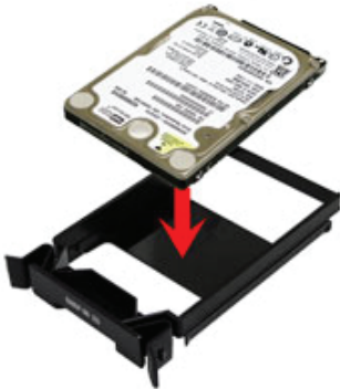
2.5" SATA hard drive being installed into Snap-In 25
