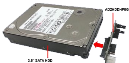
Installing the adapter onto the back of a 3.5" hard drive
