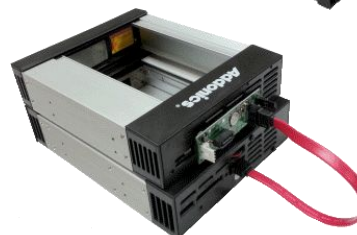
Connecting two Mobile Racks to the adapter
