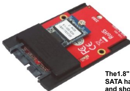
Completed assembly of the M2 -Micro SATA adapter with M2-SSD and drive frame
