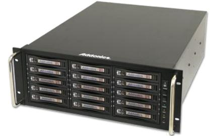
You can start your RAID Rack with as little as one hard drive and expand by adding more hard drives as your storage requirement grows. Depending on the model, the 20 hard drives are set up as 4 RAID groups that connect to the system with 4 eSATA cables or a single mini SAS cable. There is also choice of models with hot swappable redundant power supply for mission critical applications.
