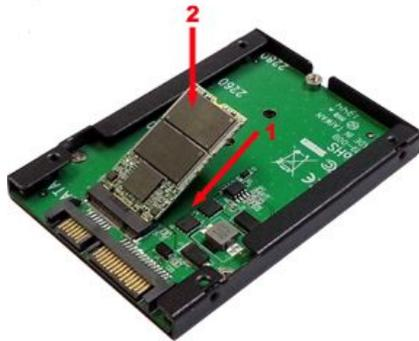
3. secure the M2 card to the PCB with the screw that comes with this drive kit
