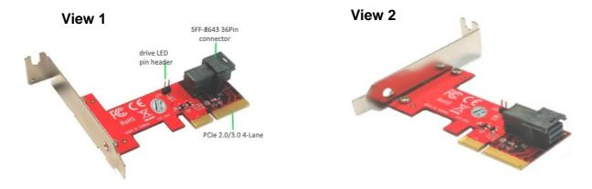
Illustration of connecting the 2.5" NVMe U.2 SSD via a SFF 8643 cable
