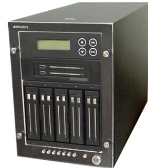
The Jasper Duplicator also offers high performance - over 140 MB/sec depending on the read/write speed of the source and target media. Whereas the performance of most duplicators declines with increasing load, the duplication speed on a Jasper duplicator remains the same regardless of number of drives in the copying process.
