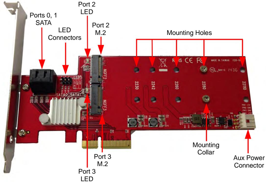
LED Connectors: “LED ALL” flashes to indicate activity on any device. LED 0 and 1 flash to indicate activity on SATA ports 0 and 1.
