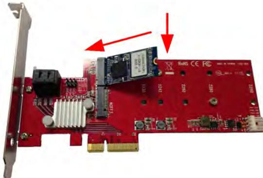
Turn the board face up again, then insert the M.2 media device into the connector at an angle, then gently press down and secure it to the mounting collar with the provided screw.
