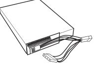
4. Connect the IDE ribbon cable to the 40-pin connector on the converter. The red edge of the ribbon cable needs to line up to pin 1 marker of the 40-pin connector. The other end of the ribbon cable will be connected to your motherboard's IDE channel.
