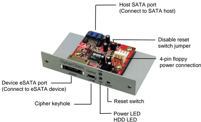
**Disable reset switch jumper** – By default, CipherChain-e reset switch is enabled. To disable reset, remove the jumper. Disabling the reset switch is recommended if the CipherChain-e is connected to a boot drive or non-hotswap SATA controller card.
