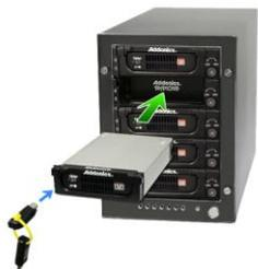
Slide the enclosure into the drive bay. Using the key provided, insert it to the lock mechanism and turn it to the "LOCK" position. This will secure the enclosure and provide power to the drive.
