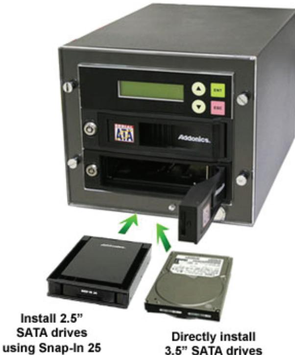
**To install a 2.5” drive into the Snap-In 25 adapter:**
