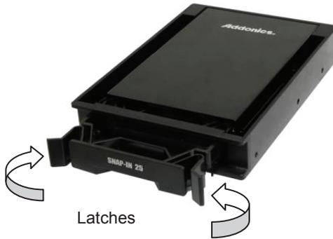
**Step 2.** Gently pull the drive retainer clips outward on the tray while inserting the drive from the top.
