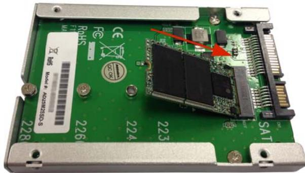
**Step 3.** Secure the device in place with the mounting screw.
