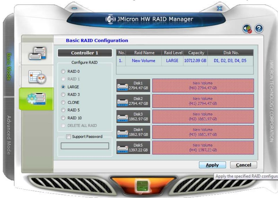
Finally, click Apply. The Jmicron RAID Manager will confirm the operation with a reminder that existing data on the drives will be lost, then perform the RAID configuration and report with a dialog box when it is complete.
