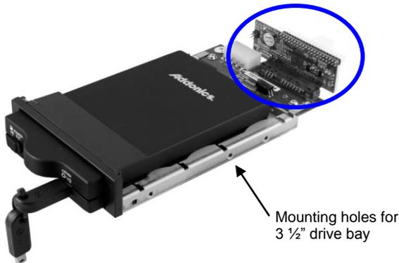
**Step 1:** Connect the 40-pin IDE ribbon cable that is connected to the IDE controller on the motherboard to the 40-pin IDE connector attached at the back of the Ruby Cipher drive cradle. This is the data connection for the device.
