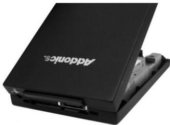
**Step 7** Lower the front of the top cover and making sure the two covers lined up properly. Tighten the small retaining screw on the front of the bottom cover to close the enclosure.
