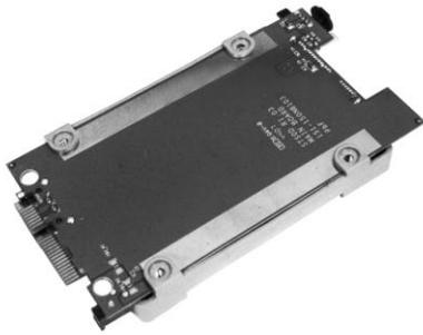
**Step 5** Mount the board to the bottom cover.
