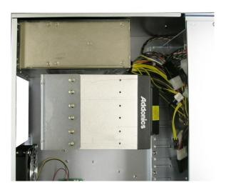
Secure the Disk array by screwing the top and bottom brackets to the frame of the storage rack.
