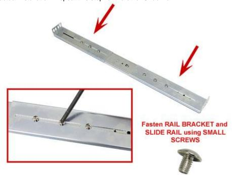
5. On the rackmount equipment, secure the L-shaped edge of the **Rail Bracket** onto one of the front rack frames, using screws included with the rackmount equipment. On the rear end of the rackmount equipment, secure the other **Rail Bracket** onto the rear rack frame. Repeat this step for the other side of the rackmount equipment.
