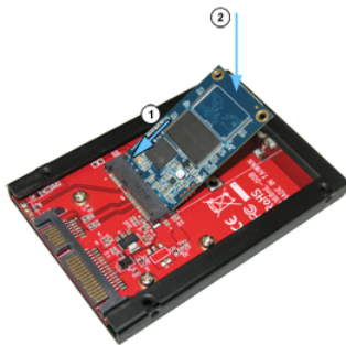
mSATA SSD installation illustration
