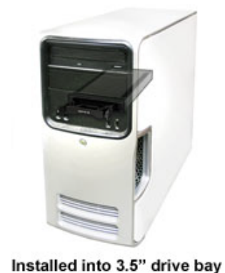
The snap-In 25 can be mounted into a 3.5" drive bay of a Desktop system
