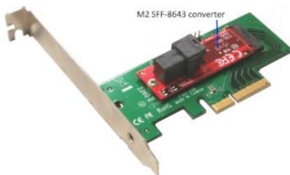
M2 SFF-8643 converter installed onto ADM2PX4
