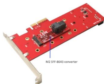
M2 SFF-8643 converter installed onto AD2M2S-PX4
