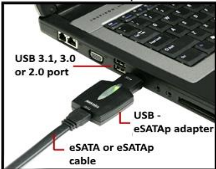
Diagram showing connection using eSATA or eSATAp cable
