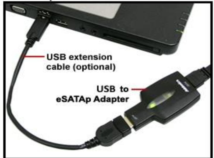
Diagram showing connection using optional USB extension cable
