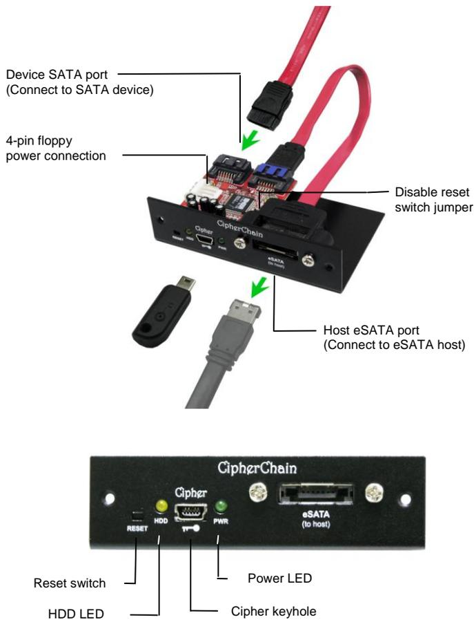
**Disable reset switch jumper** – By default, CipherChain-e reset switch is enabled. To disable reset, remove the jumper. Disabling the reset switch is recommended if the CipherChain-e is connected to a boot drive or non-hotswap SATA controller card.
