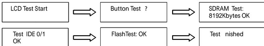
Once the system diagnostics have been completed the "Test finished" message will appear on the LCD.
