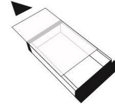
4. Carefully load the SATA hard drive into the drive tray with label side facing up. Turn over the drive tray while pressing the drive against the bottom of the tray
