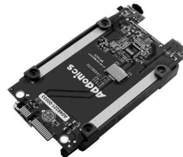
**Step 4** Turn over the PCB and secure the hard drive to the PCB with the mounting screws that come with the kit.
